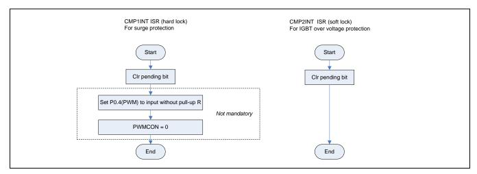
Figure 3-3 Interrupt Service Routine Diagram
